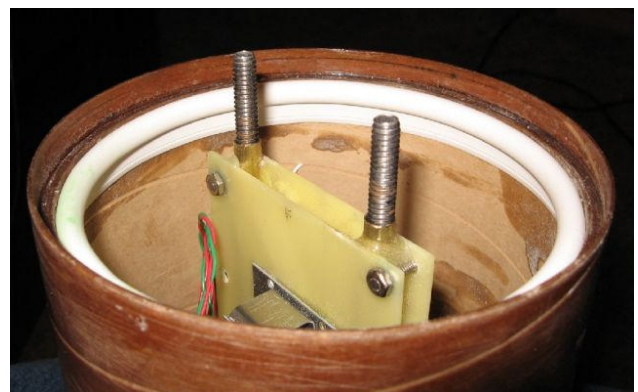
The electronics bay seal. Photo by Tim Dixon.
