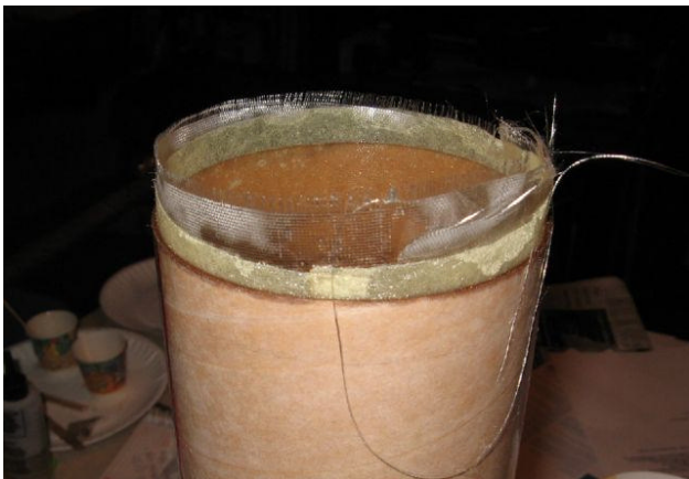
Kevlar on the forward end of the bodytube. Photo by Tim Dixon.
